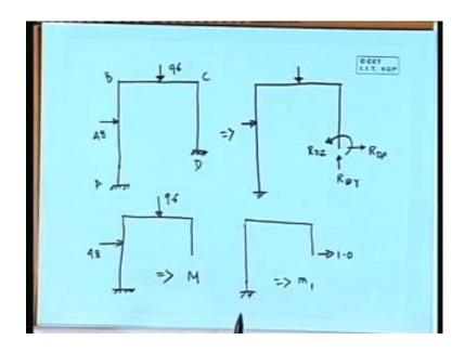
So, this is 5 meter, 3 meter, 3 meter, 3 meter, 4.5 meter, same problem; only the supports are clamped, not the hinge and the roller. The load was how much?
