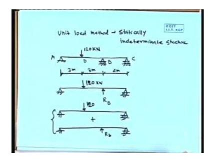
So, we can say this unit load method applied to your, right. So, statically indeterminate structure we want to solve by unit load method. Now what we can do? We can take a beam problem like this, right. So, say, this is 3 meter; this is 3 meter; this is 4 meter and the load, say, 120 kilo Newton, right. We can say this is A; this is B; it is C, and the other load it is D. So, this is a two span beam AB one span, BC another span, three supports. This support is hinge, they are roller.
