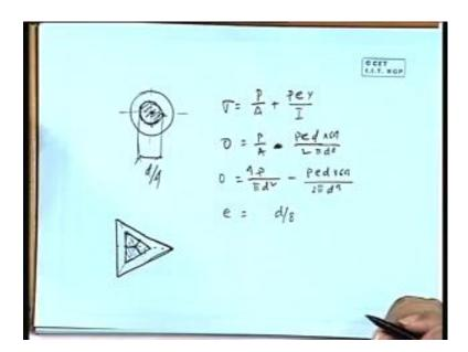
So, this is the point which is the location of the centroid if the load is here. So, it is eccentricity in one direction. So, if we just follow the approach what we have applied for a rectangular cross section with one directional eccentricity, you can find out the range of this e, so that the limiting point will be here, right. Now in a similar manner if it is here because here also it is line of symmetry. So, what will be happening? You will get a core having a circular cross section, right.
