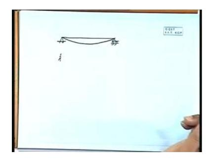
Now a simply supported problem that deforms shape is a sinusoidal form fundamental case. Now if we take a cantilever, I think I should draw in a different way; otherwise, it will not may be possible to explain; from here I am drawing it again.
