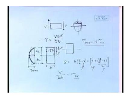
Now, if we take say this side is V; this side is V; and some cross section here. So, this cross section may be looking like this. Now, this V will be responsible for generating the shear stresses. So, shear stress it can be calculated as VQ by Ib.
