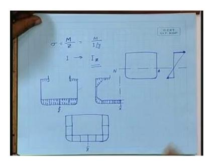
That is the section modulus gives us the bending stress. And what is this Z is basically M by I by y, where I is I at the maximum section where the maximum bending moment occurs, and y is the distance of neutral axis or the fiber from the neutral axis. Now this y can be anywhere; you can start from the neutral axis where the stress will be 0, and as you go up to the deck, you will get towards the deck what is the stress.
