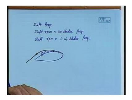
So, because of this reason, you are getting a shaft frequency excitation, you are getting shaft rpm multiplied by number of blades frequency.
