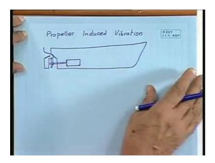
The main prime over is a propeller in a ship and from maintenance point of view, we always try to select a single propeller and therefore, a lot of power is to be transmitted through one single propeller. Usually we have 4 blades, but there is no restriction on that unless it meets our requirement.
