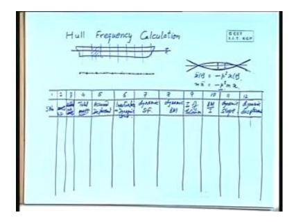
If your assumed displacement is correct and this is the mode shape, if this is the mode shape, then this and this should match; if not bring column 12 to column 5; repeat all this calculation and keep on doing this till you are satisfied. It is a very difficult job; time consuming.
