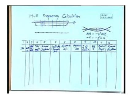
So, we will try to do. I am saying that hull frequency calculation. Now, this is a detailed method where you actually use all the design particulars of the ship. We have seen that for every section of the vessel, first of all, let us say that we have seen that hull is considered as a girder. So, when we say hull is a girder, then it is basically a beam. It is floating freely in water and therefore the end conditions are free free.
