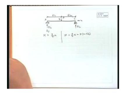
So, we took a beam like this this side some support here also, me support and centre we put P reaction we got P by 2 reaction P by 2 if we say this side is x that side this is y.
