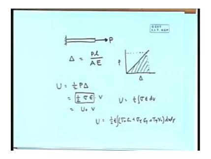
So, we took a bar in that form and applied a load P. Now, this is a case of a very simple stress problem, because entire bar will have identical stress and strength. So, anywhere stress is P by A and strain will be your total elongation divided by length of the member. So, it is a case of uniform strain, uniform stress, whatever you can say.
