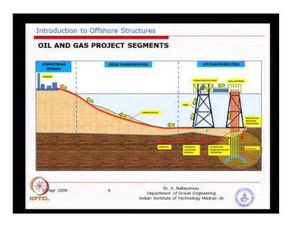
You can see there the drilling brings the oil above water using conventional techniques and then transported by out linking bridge. Normally, sometimes we see in the oil and gas development we can actually have a combined drilling cum production platform. Some cases where the water depth is larger we combine them together to make one structure instead of two structures.
