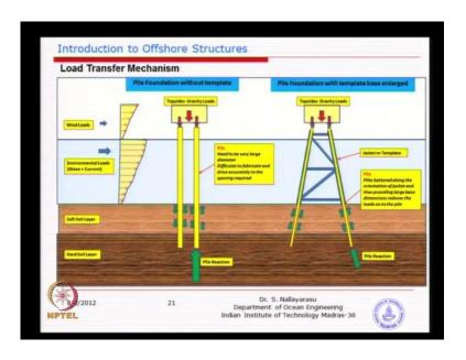
We will just focus on what exactly the idea. We were discussing few minutes back about the load transfer for fixture structures. So, that tomorrow we can move on to a new chapter. So, you see the first one conventionally a individual pile. You might see this type of construction. When you go to a coastal areas or even land you drive several piles and fix up a super structure on top. Something like this you have a cylinder system one or two or three. It depends on the load carry capacity.
