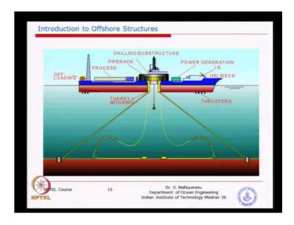
Then the F P S O of different kind you can see here have a mooring, which makes the ship to rotate about its centre of the axis. You see here there is a yellow colour bearing
