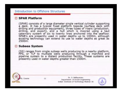
Ease of installation and cost efficiency is very high compared to other hulls. Many, times in the last twenty years almost hundreds of spar platforms have been installed in the deeper waters in seen some cases. We also have alternatives whenever the water depth is too large. Proved to be expensive to go for a floating system we come with a sub sea systems.
