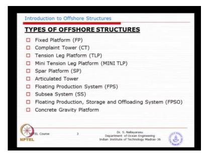
I think one by one we are going to see some pictures as well and understand the concept of how the load transfer is happening fixed platforms complaint tower. Both are based on fixed to the ground type, then the remainder is almost all of them are floating type, one by one. We will go through and the last one is the gravity platform.
