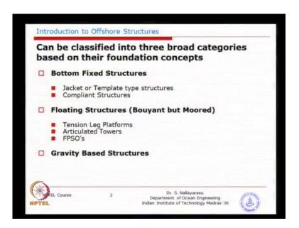
So, you have jacket or template type structures compliant structures. We will see the difference between what is a idea behind jacket structures and compliant towers. The second class will be floating structures, where the load transfer is by means of buoyancy. So, there is no foundation except for mooring lines. Then the third is gravity based
