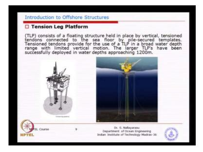
So, we have seen this earlier tension leg platform the concept is very simple. It is very similar to simple floating pontoon the load or the payload is at the top. It is floating, because you have excess buoyancy. So, you may see that if you look at that there is a horizontal pontoon is connected to 4 legs. Each of the columns is connected to the
