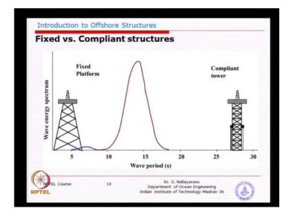
Something similar given in period fixed versus compliant. So, the most of the energy content of the wave will be about in fact between 10 seconds to 16 seconds potentially very large energy magnitude. Whereas, the fixed platforms we keep it in this side the complaint tower or floating system is going to the other side.
