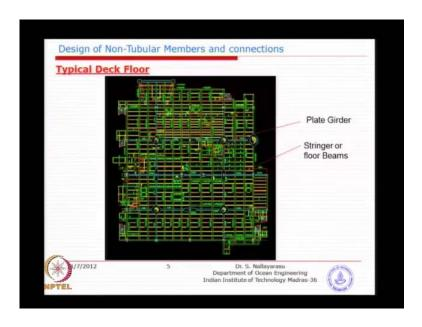
Typically, if you see this drawing this is how offshore platform floor will look like you know you this is particularly four columns structure, four column is basically one column here, another column, another column, another column. Then, I do not know whether see the colors, the blue colure is the grid beams where it should be deeper and you see other yellow color beams which are floor beams or a runner beams. You know basically supporting the equipment floor plate and facilities.
