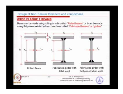
The beams can be fabricated or obtained from mills, so you can see on the left one is basically a rolled beams means there is no welding involved. That means you will take a large size piece of steel and roll it to get this shape is which is called a rolled been, but one of the problem is larger sizes are not available readily because nobody will make this kind of beams and keep it ready.
