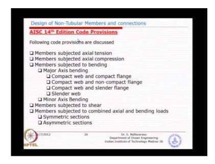
So, next class will look at what we are going to just see are the course provisions for the ASE for various forces of action on the beam, actual tension and compression bending and the shear and the combinations.
