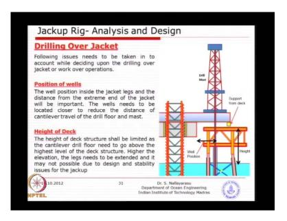
So, typically the drilling over the jacket, I think we have discussed most of the parameters. Position of wells, height of the deck I have just mentioned about each of this parameter needs to be considered a before arriving at which jack-up is for this particular site.
