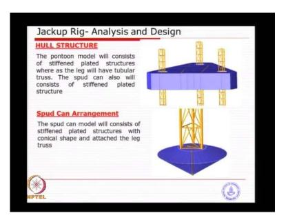
Just a close up picture of the hull and the spud can. Spud can is little complicated fabrication itself in this particular one. We had a large diameter pipe going all the way. The stiff end plates inside in some cases you may not have the central tube. This is one of the analysis for survival condition, you could see the top displacement is two and half meter during a storm condition.
