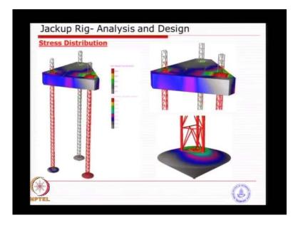
Quite a number of location you can see red colour all of them is overstressed. So, what we need is we need to strengthen the structure, because over stressing is due to additional loads introduced. because we are converting drilling rig to production rig. So, you even see here most of the leg portion is almost over stressed. So, you need to substantially strengthen the structure to accommodate the new loads. Also, the spud can connection is heavily stressed.
