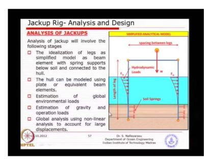
Simplified is initial stage, we try to do a simple pontoon frame analysis, not of course two dimensional or three dimensional. You can see here what we are looking at is equivalent leg diameter. You have a lattice structure, if you can come up with a equivalent diameter, because you want to look at the behaviour quickly instead of modelling so complicated structure.
