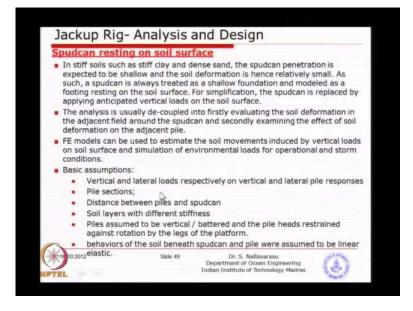
We need to look at how they can transfer because when it is laying on surface. So, that means only a frictional capacity can be available no lateral expression will be available, because it is not penetrating enough. So, in such case of basic in a spud cannot able to penetrate. Then we may have to look at various other aspects of introducing alternate mechanisms, one of such mechanism is basically provision of skirt on the spud can.
