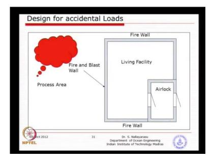
Typically, you will see a living facility will be encompassed by a peripheral fire wall most of the time because, you know basically it does two things. One is, one is the temperature reduction due to fire, the other one is heat loss, you have a air condition
