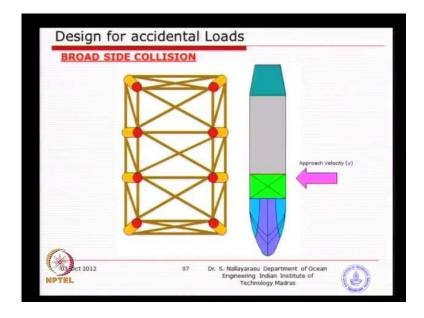
That is the purpose of which is basically to evaluate such a scenario or if it drifts in this phase and comes and get in contact with the structure in a parallel way. That means multiple contacts at simultaneously, which will be not a very a critical case because, so many legs are there, the damage could be lower than the corner impact.
