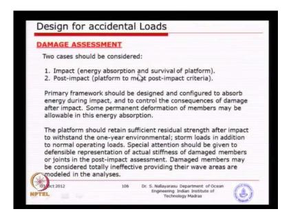
Damage assessment basic idea is the energy absorption and survival of the platform that means, you do not allow the structure to fully collapse during the process of impact. Post
