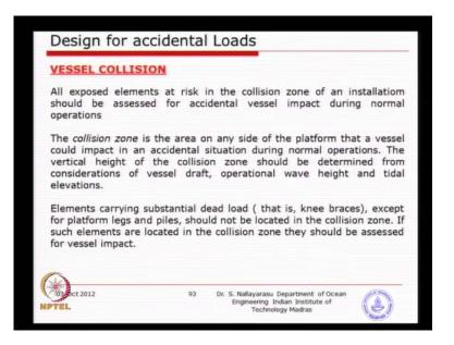
The vessel collision zone is something that we need to carefully evaluate, it is not going to hit the bottom of the structure because, the ship may not be able to go unless you have a submarine coming there. So, basically what we have is a particular zone in the structure near the water line, slightly above slightly below, which we call it, I think we have defined as the splash zone area, the change in tidal levels low tide to high tide.
