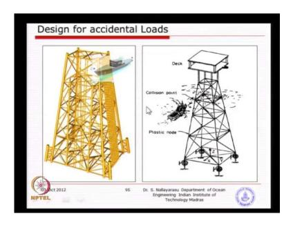
Typically if you see there in this vicinity, the near the water line you may actually see that the high potential of direct impact that means, those members only needs to be designed for such type of impact not the members below. Because, they have no axis through the boat because, the boats cannot get submerge unless, the boat itself is capsizing and then, go and dive downwards which I think it is a different scenario.
