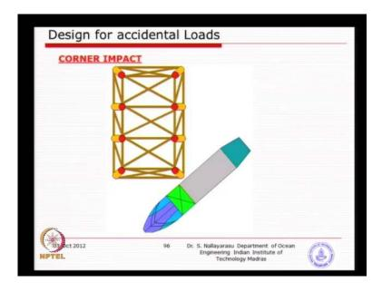
There are two or three types of impacts are expected. For example, you see here drifting vessel, engine failed, environmental conditions are deteriorating and the vessel has no
