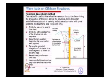
Just you see from this picture we have a vertical cylinder and the wave is progressing in a direction, perpendicular to the cylinder axis and just moving continuously. So, at what instant of time maximum force will come, which needs to be evaluated. So, what we can simply do is we can just take this Morison equation.
