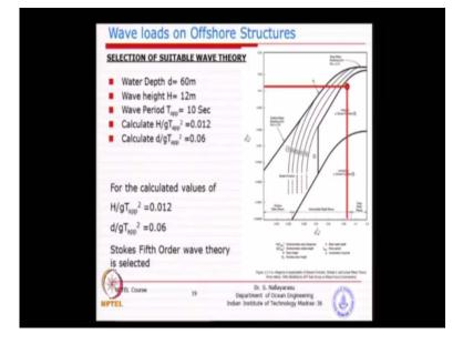
So, typical example for a location what you see here in this chart is a water depth is 60 meter wave height is 12 meters and then associated period is 10 second, calculate this both the parameters. And then you could see that straight away strokes wave theroy is applicable so for a typical jacket location of 60 meter water depth you could see that the
