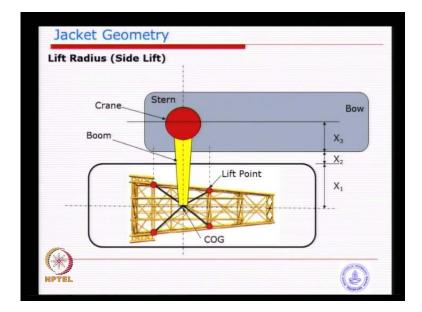
The side lift this is called the side lift, this is what you saw from the picture. The larger this distance X 3, X 2, X 1 the more trouble for the barge, so we need to design for it. As long as you can achieve this condition by means of ballasting by means of design it is fine; otherwise, we need to look for lifting in this fashion.
