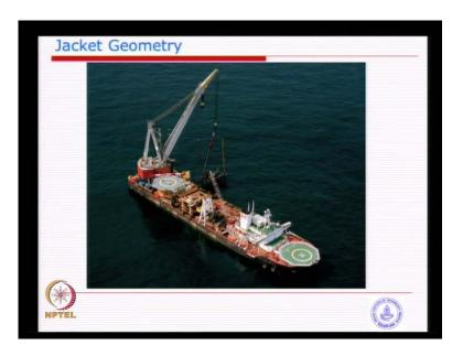
Typical crane vessel, so this is what I wanted to show you. See the crane is on one end; if you are doing a heavy lift on using this crane, you can do ballasting of the hull on the right side, so that is the idea behind. All the offshore cranes have a huge capacity ranging from few thousand tons to thousand tons to typically about 10000 tons, 15000 tons crane is also available in some part of the you know North-Sea; some of the contactors have such capability.
