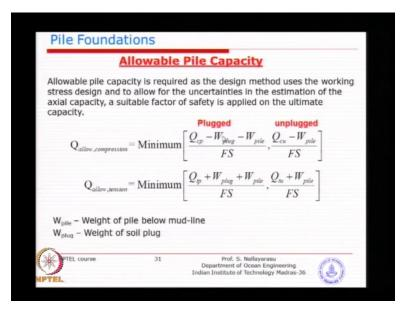
So that is exactly when it is plugged case weight of the pile plus weight of the soil must be taken out of the capacity for the buried portion, of course the portion above the sea bed is anyway part of the load because you are analyzing the jacket structure.
