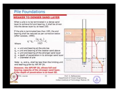
The first case if you see the this picture you have a medium sand to a dense sand transition from sand to sand but you have a slightly less dense on our first layer and a denser sand on the last layer where I have decided to penetrate into the denser layer and then bound to take advantage of the capacity.
