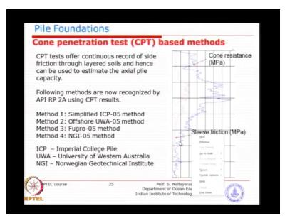
Okay, so the last week we were looking at the CPT results so typical record of measured you know the sleeve and the cone friction is given in this type of diagram so basically this will be the output from the country's recorded CPT test. So what we were looking at is the several methods of integration based on the localized in fact this the reason why so many methods are there because its (())(0:42) the empirical coefficients of different cones and basically the integration methods.
