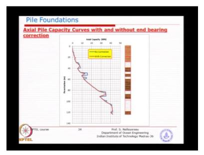
We will now look at a capacity generation for interface layers for example I have a only single layer soil of clay or sand then there is no issues, whereas when you are talking about offshore pile systems, for example if you see here multiple layers of alternating types sand and clay.
