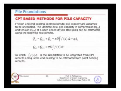
And you will see here that the calculation is very similar to what we were doing if you are having a strength profiles as layered size here we have a continuous resistance for skin friction and the end bearing and basically you are trying to two integration from the depth to depth from starting to end and you have compression and tension capacity in terms of tension capacity you do not have the end bearing, so basically it is coming out.
