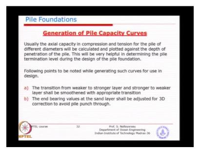
Now normally we do not know the pile penetration in a design work which we will have to calculate for several iterations when you are designing a jacket you do this analysis and find out what is a pile loads. To determine what penetration is required you are not going to do everyday calculation separately.
