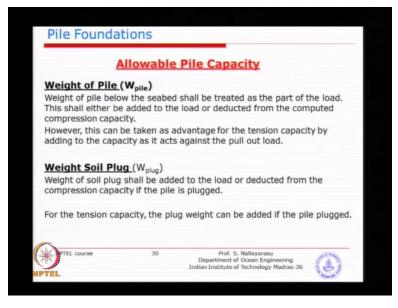
Now how do we find out allowable capacity is just a simple matter of taking the ultimate capacity divided by factor safety but then the added information that we need to remember is the weight of pile and weight of the soil plug remember we were talking about when you drive the pile inside and just pull out the pile if the pile is plugged one, what will happen the soil will come out together with the pile itself.
