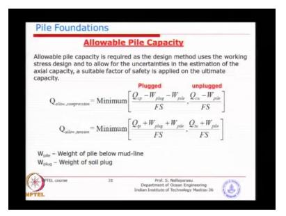
So that is there we need to make sure use this you know basically the information. In the plugged case you will remove the pile weight and the soil weight from the capacity divided by the factor safety because it is part of the load.
