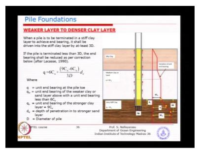
The next one is you have sand layer and a stiff clay of course arguably clay is not going to offer so much of end bearing capacity as you can see from the equation you know is undrained shear strength is the only parameter which is contributing to your end bearing which is not going to offer two grade unlike sand layer where the over burden pressure is going to present good amount of you know the end bearing resistance.
