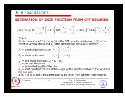
And the idea of getting this fz from the method cone sleeve friction this is the sleeve friction the red color one is to get the idea of fz, fz is the frictional resistance.
