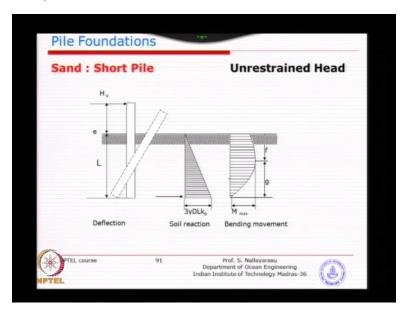
And then again we will just go into the sandy material that what we saw was is a clay then we can go into sandy material the only change is the resistance is linearly proportional to the overburden pressure so you will see a triangular distribution and that is the measure difference between the clay soil and the sandy material so reminding is behavior will be short pile or long pile and with and without the pile fixity at the top, so you will see 4 cases similar idea only you
