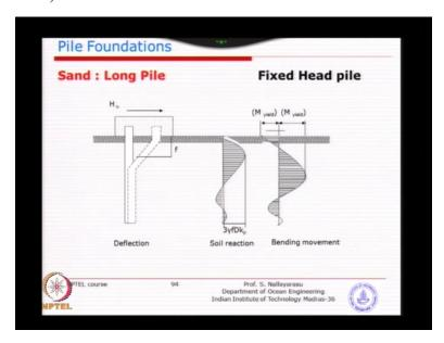
Similarly you have a long pile but still fixed headed almost you will see double locations of bending moment, bending moment maybe maximum here and because of the long pile you also have the bending moment developing at the some depth below the so all this is various limiting cases. So how do we get the general solution is we have to solve the beam on elastic foundation, so we will just look at some of these cases.
