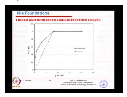
So only assumption here instead of using a nonlinear spring Vesic has given a quick solution that the iteration becomes easier because every time you are going to do a linearized if you go back to this picture you will go through this line rather than this line.
