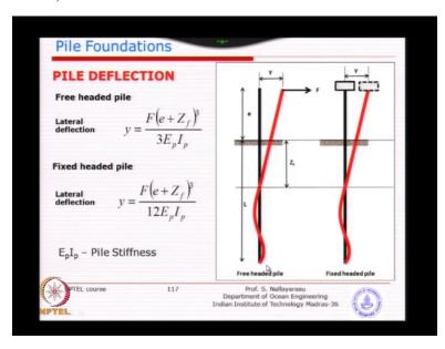
Pile deflection I think is a similar derivation which we were using earlier on you know solving the beam and elastic foundations the deflection at the pile head is quite important because when you are looking at the depth of fixity that is there you are worried about you can substitute this and find out whether your assumptions are correct. (Refer Slide Time: 41:06)
