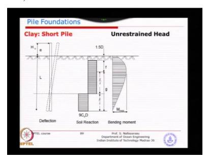
In the last one we were seeing is this the short pile and unrestrained head this is the case mostly you will encounter in offshore or costal applications where there is not much a big structure at the top you may have a structure but is not going to as rigid as onshore structures where we have a very big building with a pile cap restraining the pile foundation moment.
