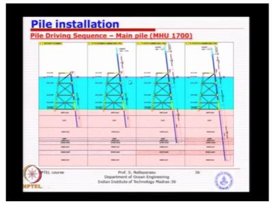
Slightly bigger hammer, skirt pile of inclined say same business the only difference is the portion of the pile will be removed. So how do we do it because this is outside skirt pile of inclined nature the last segment of the pile will have to be removed it is not permanently required, whereas in the main pile case it is permanently inside and it is going to be grouted,
