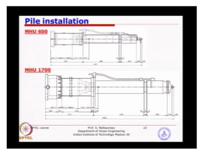
Typical hammer, so you can see all those hydraulic pipes the inlet and the outlet, anvil, housing and all those components typical number I can see 19 meters if you read it carefully is about 20 meter, this is one of the biggest hammer in offshore industry. So 20 meter long imagine it is quite bigger in size if you have a 100 meter pile, 20 meter long hammer and the weight is this particular hammer is nearly about 180 tons.
