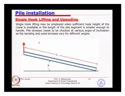
Lifting specially the longer segment piles, you see here these picture you could lift only at the end 100 meters if you try to lift from one end something like this picture you will see that the slenderness I think you could easily understand what will happen to the allowable axial stress the longer the allowable axial stress will be very very small.
