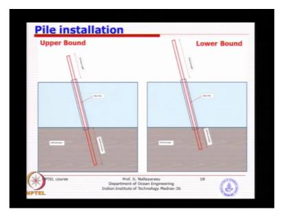
So you can see here this is what we were trying to discuss. So pictorially you can see upper bound, lower bound, stickup versus self-penetration is exactly opposite. So upper bound you see the larger self-penetration, lower bound smaller self-penetration but the same pile provides you with upper bound stickup for the lower bound self-penetration, so just opposite because of the same pile that is getting penetrated to into the leg as well as to the soil.
