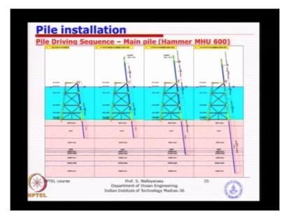
Finally we will just look at some of the sequence sketches how things are done in specially driving (())(37:16). So you can see 1, 2, 3, 4 pictures, so you have placed a longer section of the length of the pile in such a way that small length of the pile is sticking above jacket, you do not want at that time bigger length. Then you bring the second length of the pile weld it on top of the first one which is little bit sticking up.
