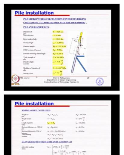
One example I have given you for so that you can go through it is also including some stress calculations based on you know our previous design course with all the slenderness ratio and allowable axial stress, allowable bending stresses which you should be familiar.
