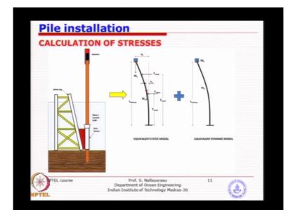
Even otherwise if you are able to do that handling and after you place this pile inside the sleeve like what you see in this picture, this is the skirt sleeve which is nothing but a large diameter pipe attached to a jacket you know and you insert this pile. Once the pile is inserted because of the weight of the pile it is going to penetrate the soil which is weaker in the last few meters of the top layer and because of that it will just start to go down.
