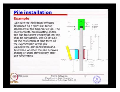
So one of the example that I have just compiled here you could go through when you get the slides is a typical water depth of 60 meter and the current is around 3 meter per second which is in the west coast northern west coast I would say and then you have a Cd value is given. So you need to find out the self-penetration which is very easy to find out a self-penetration is potentially a simple bearing capacity problem.
