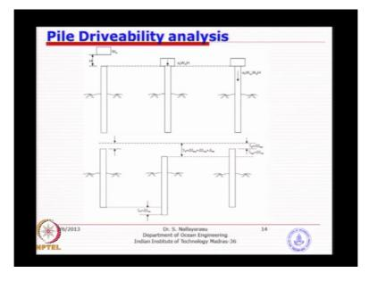
So what you can see in these picture is starting from the pile is into the ground at certain level after through you are just analysing it or you could actually have the pile just resting on top of the sea bed and trying to drive and dropping from a height of H with a weight of W h which gives you the impact energy is basically the weight times the height and energy efficiency of the hammer itself the internal system, how much it is 90 percent or 80 percent depending on what.
