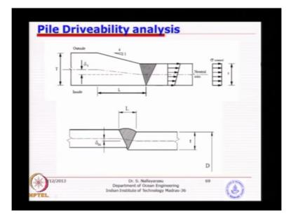
Typical detailing that we need to just look at what causes the failure, so if you look at this picture you have a thickness 1 on this side, probably smaller thickness and the bigger thickness and we wanted to keep one of the face as fresh that means the either the inside this particular case the picture shows the inside is made fresh that means the diameter is constant throughout and you have access to welding from only outside. When this will happen? This
