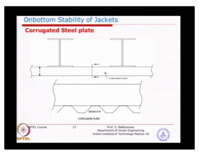
Or you can use a steel plate in a corrugated shapes very similar to propiled steel plates, this gives you additional strength instead of this kind of flat plate, you know the bending strength is very much small so you would require considerable support stiffening rather than we use a corrugated plate you know automatically we can span for a longer distance so that is something...
