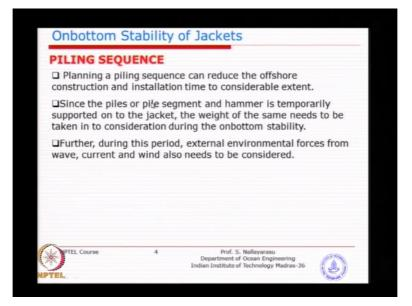
So this piling sequence is something that we need to arrive based on the COG of the jacket, sometimes some of the jacket's COG is towards one side, in such a case you better avoid going and placing a pile on that particular location. So planning a piling sequence actually
