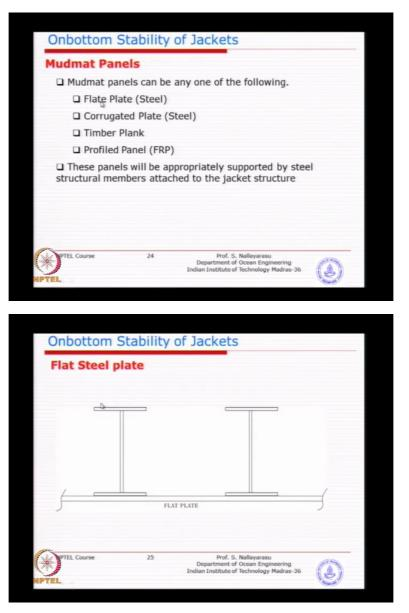
So steel plate we can use a flat plate or you can use corrugated plate, so this is the flat plate you can see the plate is attached to the bottom of the jacket.
