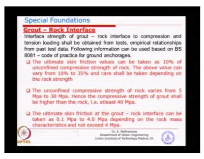
So we have seen this rock grout interface, the only information that is available for us is BS 8081 API does not give any guidance on the grouted steel pile or grouted rock interface, no
