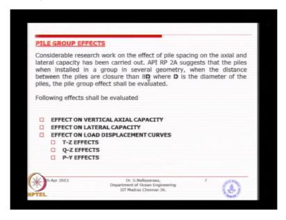
So 8 diameter suggestion means if you are able to maintain spacing like that maybe we can ignore but otherwise if you have less than that then you look at each one of the aspect and look for reduction in the capacity, so far we have already worked out axial capacity means of skin friction, means of end bearing and also lateral capacity 3 things we have already worked out. 3 displacement relationships also we have worked out basically TZ, QZ and then PY.
