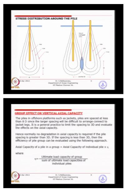
Now in this load goes down the soil and then the soil is loaded and as shown in earlier sketch, some part of this below the ground is going to be loaded twice, so basically that and when you try to fill this soil, some failure pattern will come for each file and it is going to fail together. If you keep this pile very close, what happens is classification of the soil in this zone between the 2 pile is going to be very fast compared to this soil outside, so what happens is
