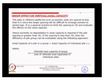
So let just quickly start with what is the axial capacity effect? So normally if you look at say 2 piles, the pile is circular section and installed at a specific spacing say 2 diameter, 3
