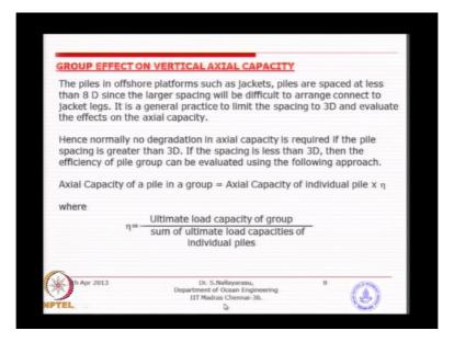
So basically that is the idea behind the ultimate group capacity has to be established by somehow, either the way that I have explained or you do an experiment or you do other means of evaluation and basically the individual capacity also easily can calculated by soil engineering friends or by other means.
