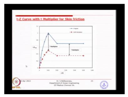
Similarly for TZ curve for T multiplier is basically you see here the original graph is the blue one whereas the reduced capacity for the same deflection is this much, so we are just having the same capacity scaled deflection to a same level and only the capacity is reduced.
