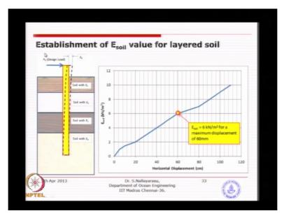
Similarly when you are applying horizontal load you could also need to find out apply the loads and incremented whichever steps and then plot with respect to this will give you horizontal soil modulus for use in your modification work and mostly if you see something similar what we are looking at piles soil interaction soft base you can apply load in various steps, obtain the displacements and plot this type of relationship to get the E value.
