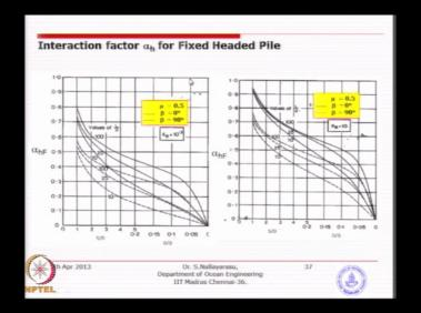
And then seems to be same or different seems to be same this is free headed piles, this is fixed headed piles so there will be another repetition of 3 more graphs. Mostly you will need to read the fixed headed piles because for offshore steel type jackets were the pile head is connected to the jacket leg you will not be able to treat it as a free headed pile unless you
