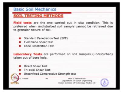
So standard penetration test is one of the best method for shallow bore holes and where you cannot bring undisturbed sample, especially whether if the soil is too soft or if the soil is fully coarse-grained, you know you could pick up the undisturbed sample, this will be the best method which can be adapted. The second method is the vane shear test, is again, is a very simple, imagine you take a Spade and insert it into the ground and try to rotate the Spade, you
