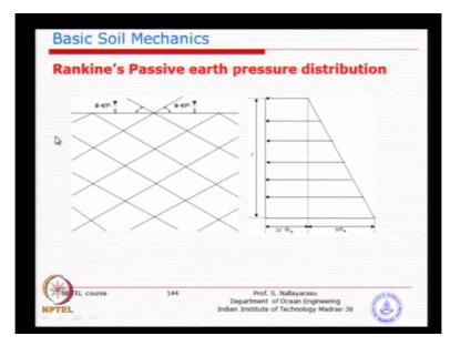
Except that you are going to see plus here because it is changed the other way around. So you can also substitute similar and the relationship you see here the passive earth pressure is vertical component plus the cohesive component which is similar picture you can see in the diagram. This failure plane is 45 minus phi by 2 because it is shallow and you can get the distribution of the passive earth pressure along the depth.
