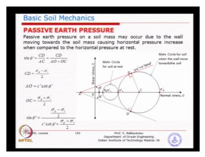
Basically you can plot the coefficient or you can plot the pressure. Similarly we could derive exactly same procedure only thing is in this case horizontal stress is higher so passive earth to earth pressure or the soil is the pressure applied on the soil by the movement of the wall is more so sigma B becomes larger and sigma V becomes smaller , so that's why the soil is able to move.
