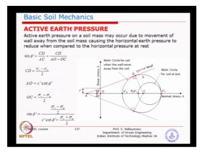
So basically what you see here is the you know the state up stress in a two dimensional space, horizontal stress vertical stress, and using Mohr circle you try to derive the relationship between the property so called you know the angle of internal friction and the intercept which is basically this cohesive component of the c5 type of soil.
