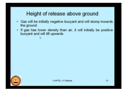
Height of release above the ground also matters in the dispersion models. Gas will be initially negative buoyant and will slump generally towards the ground. If the gas has lower density than that of air, it will initially be positive buoyant and will get lifted upwards.
