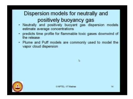
Dispersion models for neutrally and positively buoyant gas. Neutrally and positively buoyant gas dispersion models estimate average concentrations. They predict time profile for flammable toxic gases downwind of the release. The plume and puff models are commonly used to model the vapor cloud dispersion. In the next lecture, we will see in detail about these models.
