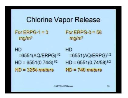
I can also do this exercise for ERPG-1, which is about 3 milligram per cubic meter. And I get hazard distance as 3254 meters. If you do for ERPG-3 level of 58 milligram per cubic meter I get hazard distance as 740 meters. So, we have got two examples solved - one is for a liquid release, other model is for a vapor release.
