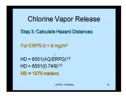
Based on the CEI value obtained for different ERPG levels, I compute what we call as hazard distances. Obviously, as a standard as for ERPG-2 level, the hazard distance given by this equation as explained in the previous example. The hazard distance is known to be 1.878 kilometers.
