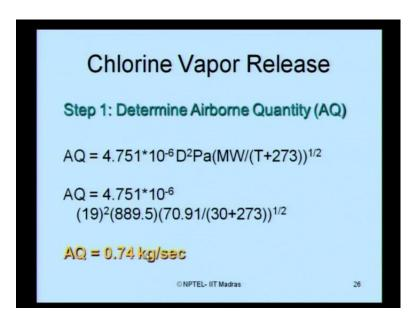
In step number one, I try to estimate the airborne quantity. The airborne quantity is given by for a chemical vapor release is given by this equation. So, I know after substituting for D as nineteen, as P absolute as 889.5 and molecular weight and the ambient temperature of the operation; I compute airborne quantity as 0.74 kilogram per second.
