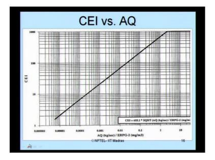
This curve clearly tells us the chemical exposure index versus airborne quantity for different ERPG values. So, if we look at the variation of airborne quantity in kilogram per second for ERPG-2 expressed in milligram per cubic meter. For a different values of AQ varying from zero point five zero(s) of 1 to 10, then obviously, the chemical exposure index number keeps on linearly increasing in this curve.
