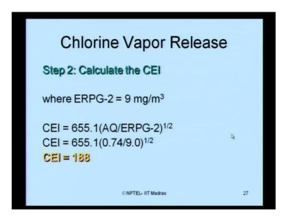
After finding out that is a step number two, I will directly compute as what we call as CEI. For ERPG-2, for chlorine vapor available in the literature is about 9 milligram per cubic meter. The CEI is given by this equation as we saw in the last example as well; I substitute the values and I get CEI as 188. It is a simple number.
