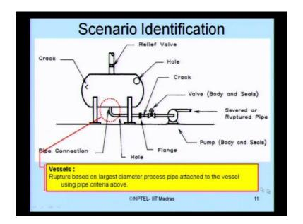
If you look at the connection failure at this junction then the rupture based on the largest diameter in the process pipe attached to the vessel should be considered for the analysis.
