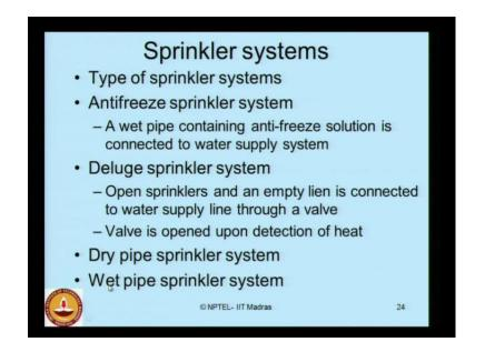
Lastly, when we talk about the effective control of fire accidents and prevention, we can also design what we call as sprinkler systems. Ladies and gentlemen, you must have seen a very common sprinkler system being used for gardening in large areas. Nowadays, under HVAC regulations that is heating ventilation and air conditioning regulations for controlled space in any multi-storey building; sprinkler systems are mandatory for fire protection devices.
