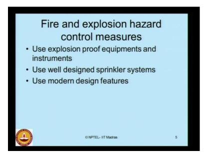
There are many hazard control measures related to fire and explosion. Use of explosion proof equipments and instruments are strongly recommended as one of the effective hazard control measure for fire and explosion reductions. You can also use what we call as well designed sprinkler systems which we will discuss in the current presentation. You can also use modern design features which we will just give a brief summary of some of the tips about the modern design features.
