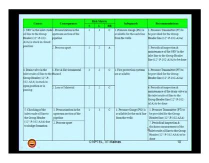
Let us look at the further cause, cause number three. Non return valve in inlet line on the oil group, it can result in pressurization of the upstream section, it can also safeguard is there using a pressure gauge, but we recommend to provide a pressure transmitter and a period inspection of and maintenance of non return valve.
