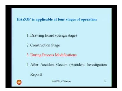
Let us quickly recapitulate that HAZOP is actually applicable at four stages of operation. You can apply HAZOP at the drawing board stage which we call as a design stage. You can also apply HAZOP at the construction stage or the process stage. You can also apply HAZOP when you want to make any process modifications or finally, you can also do an HAZOP study once the accident has occurred. We specifically call this kind of action as accident investigation report - AIR.
