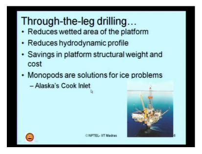
It reduces wetted area of the platform; reduces the hydrodynamic profile and savings in platform structural weight and cost. Monopods are one of the solutions, which are generally employed for ice problems. The picture what you see here is Alaska's Cook Inlet monopod platform - which is being employed or catering ice problems.
