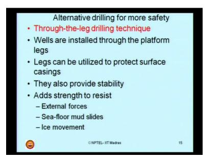
Can we think of alternative drilling for more safety? The answer is yes. There is a recent develop technique called through-the-leg drilling. This can be seen as an alternative
