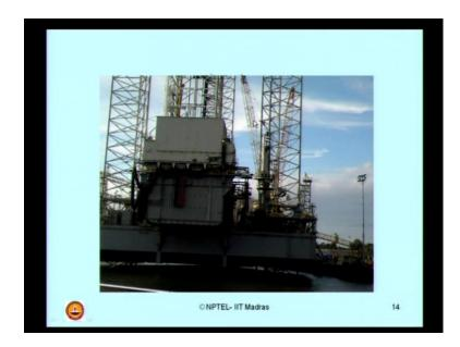
This is another picture of g s f magi lane jack up rig very famous and very common type of jack up rig deployed by the drilling fleet.
