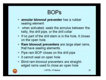
The annular blowout preventer has a rubber sealing element. When activated, seals the annulus between the Kelly, the drill pipe, or the drill collar. If no part of the drill stem is inside the hole, it closes on the open hole. While the ram blowouts preventer are basically a large steel rams that have stealing elements. The pipe ram BOP closes the drill pipe; it cannot seal on open hole of course. The blind ram blowout preventers are straight edged rams used to close an open hole.
