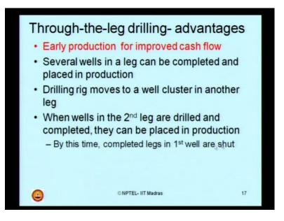
Through-the-drilling process has couple of advantages. It leaves to early production for improved cash flow. There are several wells in a leg that can be completed and placed in production. The drilling rigs move to a well cluster in another leg. When the wells in the second leg are drilled and completed, they can be placed in production - by this time the completed legs in the first well are already shut.
