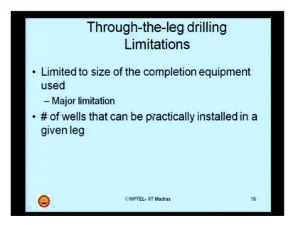
Of course, this process has certain limitations. It is limited to the size of the completion equipment used; it is considered as one of the major limitation in drilling process. The number of wells that can be practically installed in a given leg, is also one of the major limitations of this kind of drilling process
