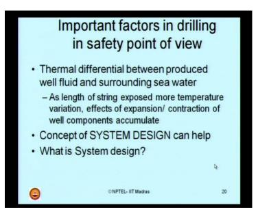
Let us quickly look at the important factors in drilling in safety point of view. There exist, the thermal differential between produced well fluid and the surrounding sea water. As length of string exposed to more temperature variation, effects of expansion and contraction of well components get accumulated. How to solve this issue? Now, in the recent development of drilling people introduced what is called system design concept. Now what is a system design?
