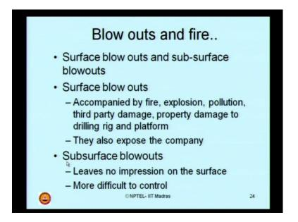
Let us quickly look at the safety during operations. Take again an example of drilling. When we talk about safety during operation, the major terminology which comes into play, is blow out and fire accidents. Blow out accidents and fire accidents or if it all occurs in drilling operation, are considered to be highly catastrophic.
