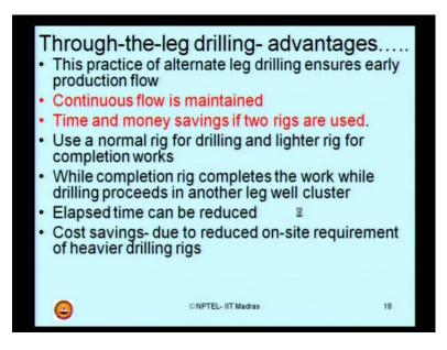
This practice of alternate leg drilling ensures early production flow. Further, continuous flow is also possible, time and money savings, if two rigs are employed. Use a normal rig
