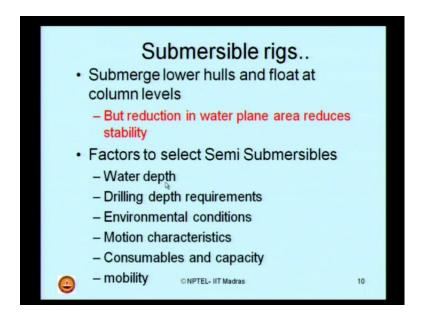
Now what happens, if you reduce the water plane area, submerge the lower hulls and float at a column level? This is how you can reduce the water plane area, but reduction in water plane area reduces stability of risk during operation.
