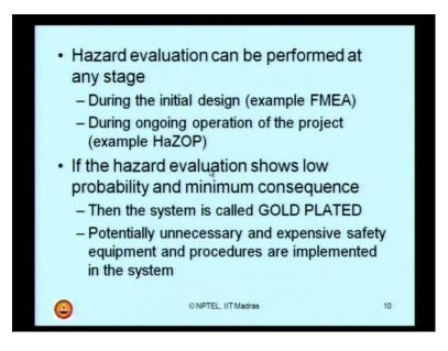
Now, hazard evaluation can be performed in any stage in the plant. For example, you can do this evaluation at the initial design stage itself. For example, FMEA is one such
