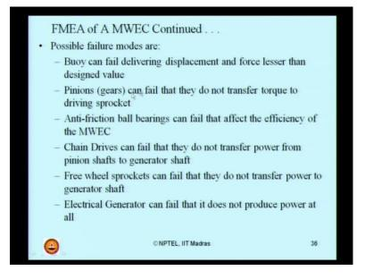
What are the possible failure modes? The buoy can fail delivering displacement and the force lesser than the designed value. The buoy may not give you a designed force; therefore, there is no design output in the generator - that is one possibility is a failure.
