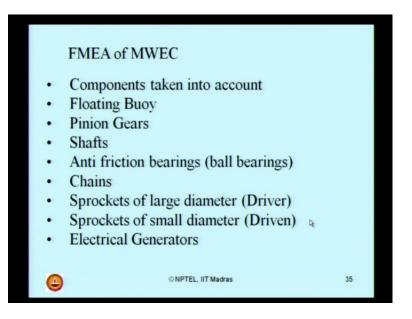
Let us identify now slowly the components, which component will you taken to account. I can list the components, I will give a past time of few second. Can you write down the list of components, which you now consider for an FMEA analysis of this mechanical wave energy converter.
