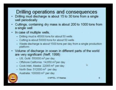
Now let us look at the drilling operation and the consequences of this as marine pollution. The drilling mud discharge is about 15 to 30 tons from a single well which happens periodically every year. Basically it arises from the cuttings, containing the dry mass which is being re-circulated back to the ocean environment which is to a tune of about 200 to 1000 tons from every single well which is being used for drilling operation.
