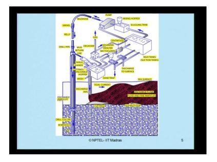
This is a very interesting conceptual figure, which explains the drilling fluid handling system. If you look at this conceptual figure in a simple format the drilling fluid is pumped inside and it pumps out lot of residuals as a reverse process. These residuals are processed and then discharged at different stages here. So, drilling as such is a process which discharges lot of pollutants in the marine environment.
