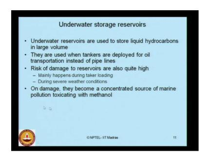
The other major source of marine pollution which arises from offshore gas and oil production platform is underwater storage reservoirs. You may wonder why we need under water storage reservoirs after all in the original source? The under water reservoirs are used to store liquid hydrocarbons in a very large volume. They are essentially used when the transportation occurs through containers and not through the pipe lines. If you
