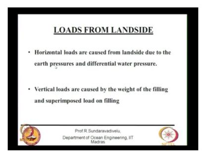
Loads from the land side are caused by the active act pressure and the differential water pressure the vertical loads are caused by the weight of the filling super imposed load on the filling. So from the land side you can have both horizontal loads as well as vertical loads. Horizontal loads are due to earth pressure and differential water pressure. The vertical loads to the surcharge load that is coming on the filling and super imposed load on the filling.
