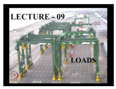
We will go to the next part of the lecture, this is one of the very important lectures which you have to study which is on the loads, what you are seeing in the figure is the containers packing yard where we have the tier mounted cranes which are used to stack the containers at different locations this is far away from the berth this is a stacking yard what you have to design.
