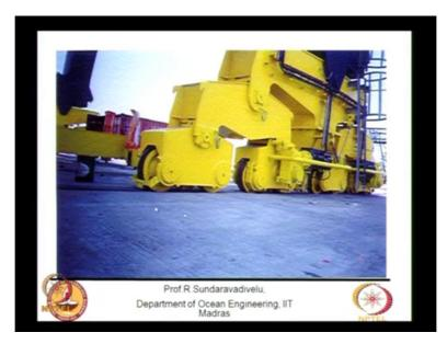
So it moves on a truck that is what is shown here and tyres. This shows the close-up view of the container crane moving on the rails is not a Mobile harbor crane it is called as a key crane. This is one leg of the crane, so we have two wheels here like that we have assembly of 4 such units. So totally we have 8 wheels.
