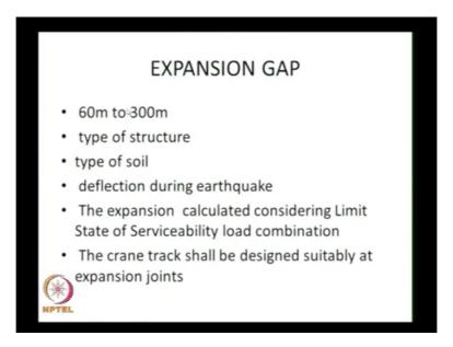
Another important parameter is expansion gap. This expansion gap varies suppose you have a 300 meter long structure, some places like Tuticorin we have built without any expansion gap at other locations at every 60 meter intervals you have to provide the expansion gaps and depends on the type of structure there is a open type structure or a solid type structure again it depends on the type of soil for a length of 300 meters if you make 5 bore holes each 4 holes give a different type of soil.
