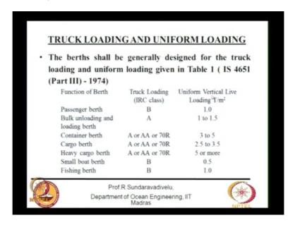
The truck loading this is given in IS 4651 there are two types of loads one is called the IRC plus, what is IRC? Indian Road congress then you have uniformly vertical live load. So depending on the classification of berth you can classify the berth as passenger berth, bulk berth container berth, cargo berth, heavy cargo berth, small boat berth, fishing berth.
