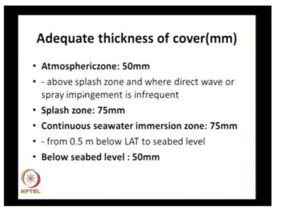
Then the cover also depends on 3 zones I am sorry 4 zones, one is atmospheric zone that is above the splash zone and where direct wave or spray impingement it is in frequent that is slightly above the high tide level that is atmospheric zone. Splash zone is where there is a water level variation where there is a wave splashing where the cover should be higher, when there is a continuous sea water immersion, we can put 75 mm from 0.5 meter below lowest astronomical tide to the sea bed level.
