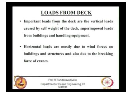
Load from the deck important loads are the vertical loads. These are caused by the sulphide of the deck super imposed loads from the buildings and handling equipment and this also consists of horizontal loads they are mostly due to wind and building and structures and also due to breaking forces of cranes.
