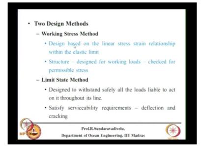
There are two methods which are used for the design one is called as a working stress design another is called as a limit state design. Earlier people are using working stress method, now days they are using limit state method. This design is based on linear stress strain relationship within the elastic limit. The structure is designed for working loads checked for permissible stresses. So I request all of you to go through this slide.
