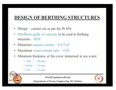
And there are certain provisions that you have to follow mainly the design has to be carried out as per IS 456 discuss in the next slide about the type of design which will carry out. The minimum grade of concrete is M 30, 30 means 30 mega Pascal is the compressive strength of concrete cube, minimum cement content should be 400 kg per cubic meter 50 kg is 1 bag of cement minimum 8 bag of cement it can be more than this, it should not be less than this least you ensure the durability.
