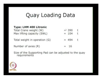
So this is called as one typical crane LHM 400, the weight of the crane is 390 tons about 400 tons it is to lift a cargo of 100 tons. If you want to lift about 100 tons the weight of the crane required is 400 tons. So the total weight is 494, so it moves on a axle that is about 16 axles then it when it is operating the four pads are lowered, all the tyres are lifted up. That time only you have the maximum loading.
