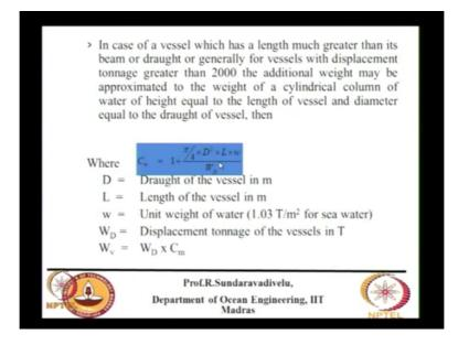
It is a larger vessel you have to use this formula it is given here pi by 4 D square L into w L divided by the displacement tonnage of the vessel, so this gives the ratio. So added mass of the vessel for I do not know whether this is correct or not. I thought it is 20000 tons it may be wrong I will check and let you know. For vessel greater than 20000 tons the additional weight.
