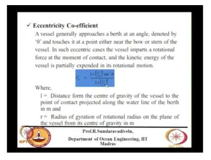
So I will not get into the theory it is very simple only theta is the angle L is the that whether it is quarter point berth and all or is the ya radius of ya we are giving because the vessel is rotating about the z axis. The energy is spent by the rotation. So the ya radiation of gyration comes into picture.
