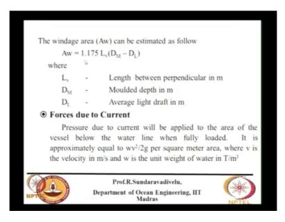
So this is for the vintage area this is depth moulded and life draft. So depth moulded is full depth and depth less average life draft then the current force is calculated w v square by 2 g where v is the velocity of current in meter per second w is the unit weight of water. Typically the velocity of the current in tidal flow is between 1 knot to 5 knots. Generally it is between 1 and 3 more than 3 very difficult to design. So this is your f c and this is your f w.
