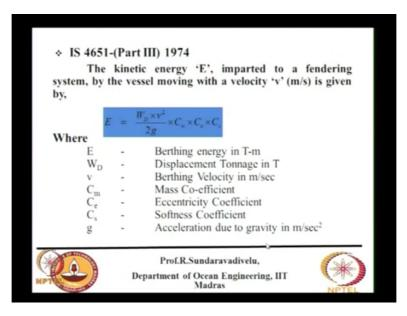
So this is the equation what you are doing that is energy is equal to w d that is displacement tonnage v is the velocity G is the acceleration due to gravity, C m is the added mass coefficient, C e is the Eccentricity coefficient and C s is the softness coefficient. So you have to find out this coefficient to get the value of energy.
