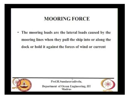
The mooring force are calculated these are the lateral loads is crossed by the mooring lines when they pull the ship into or along the dock or hold it against the forces of wind and current.
