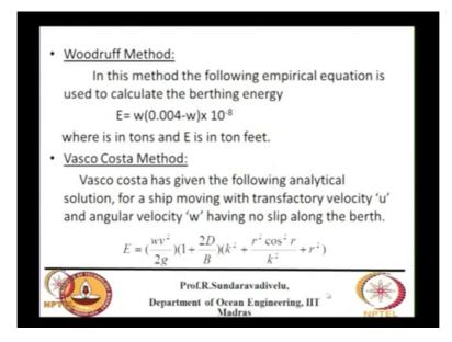
But you cannot do it here. This is most commonly used method this is analytical solution based on first principles there is a derivation for this to get this energy equation. Our IS code is using this equation to give the various parameters but if you want to know the background for the IS code formula you have to go through this there is a general paper where they have given, how they have derived the formula for this?
