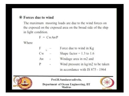
So it is given here the wind force is calculated using this formula using some coefficients the windage area and the pressure. The pressure is to be taken from IS 875. I will give a calculation, how to use this formula? So windage area is area of exposed to wind.
