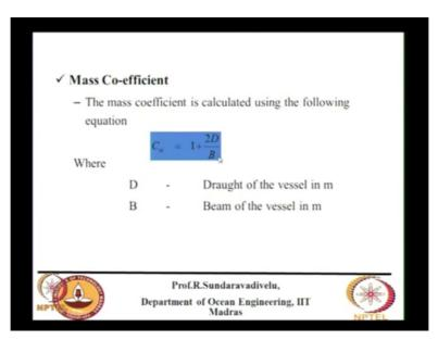
So the mass coefficient you can calculate using this formula 1 plus 2 D by b where D is the draft of the vessel b is the beam of the vessel but this equation is only valid for smaller vessels.
