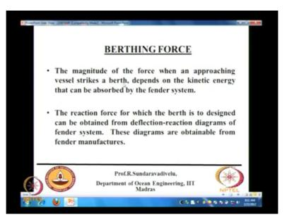
So this reaction force what I discussed this can be obtained from the deflection reaction diagrams of fender system. And these diagrams are obtainable from fender manufacturers.
