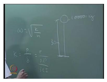
So you have seen the water tank you have a mass at the top, and the height let us say about 20 meters designed for unlock 100000 litre, 100000 litre means 100000 kg mass. Have you seen water tank in IIT campus? hmm? Where are the water tanks. Near? Jamna hostel, Jamna hostel then hmm? BSB complex so the (())(28:31) is something like this. it is a single tower. BSB only you are telling no? It is like this. Height will be 20 metres or more? Take it as 30 meters.
