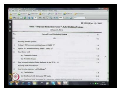
So if it is ordinary R c moment resisting factor frame this is 3 special frame means it is 5. Steel frame with a concentric braces 4, Eccentric braces 5. This macentry wall under 1.5 very low and reinforced is 2.5. So this is the intensity which you have to see, if the uniformly distributed floor load is 3 kilo Newton per meter square then we can take 25 percent. If it is more than 3 kilo Newton per meter square it is 50 percent.
