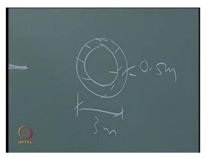
I means you have to find out this is a shaft when you take the section of the shaft like this may be 3 meter in diameter thickness may be about 0.5 meter or something like this. So from this you can calculate the moment of inertia we substitute k here m here. What is the unit of this, this will be kilo Newton per meter mass will be kilo Newton per meter per second square. So if you this will be 1 by second.
