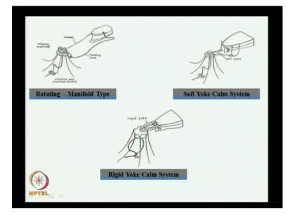
We have different types of yoke. This is called as manifold type. This is called as soft yoke. This is called as rigid yoke and these are certain classification. This is a submersible buoy, this is the hose, this is a riser pipe and this is going down vertically so that no tension is applied at this particular point. So this is normally how it is done in a riser pipe.
