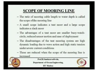
So this I already discussed, ratio of mooring cable length to water depth is called as scope of the mooring line. It is a very small, then it includes taut mooring and if it is a large scope, it indicates a slack mooring line. Advantages of taut moor are smaller buoy-watch-circle, reduced sensor motion and ease of deployment. So when there is a buoy, the buoy will move. The movement if it is less, it is better for certain applications. That will happen if it is a taut moor.
