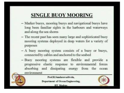
The single buoy mooring system, this can be used as a marker buoy for navigation channel and mooring buoys and navigation buoys. These are in harbors and waterways and along the sea shore. So nowadays we are seeing large and sophisticated buoy mooring systems. These are deployed in deep waters for variety of purposes. This buoy mooring system consists of a buoy or buoys connected by cables and anchored to the seabed.
