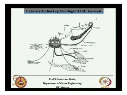
This is a single buoy mooring system. What you see here is an attachment to the single buoy mooring system which is used to connect the anchors. So in this figure we have, there are about 6 anchors. These anchors, I am sorry, 6 chains, mooring chains. These are the anchors. I am sorry, these are the anchors, this one, this one and this one. So this is a mooring chain connected to an anchor.
