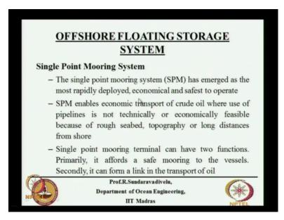
Then we will talk about this single point mooring system. We call it as offshore floating storage system because we are storing the oil in the mother vessel or permanent tanker. We call this as SPM. This enables economic transport of crude oil where pipeline, use of pipeline is not technically or economically feasible because of rough seabed, topography or long distances from shore. So sometimes we use SPM with pipeline also but in general for a loading terminal we do not use with pipelines.
