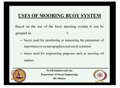
So we can group this buoy mooring system into two categories. One is for scientific purpose, another is for engineering purpose. Scientific purpose is for monitoring or measuring the parameters of importance to oceanographers and naval scientist.
