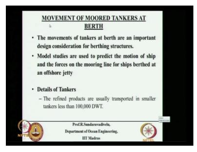
One of the main requirement of this open sea facility is what is a movement of moored tankers at berth, this I have given only for tankers. It is different for different type of vessels. It is different for container vessel, is different for bulk carrier. It is different for smaller size vessels, is different for bigger size vessels. So I will not be able to cover the entire thing but I will tell you for tankers what will be the permissible movements.
