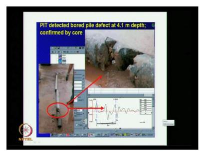
So this shows one pile which was tested. This is the total length of the pile and this will be the first signal, this should be the second signal. So you are showing the problem somewhere here in the record and they have excavated the pile. Then you are seeing how the pile is. So this defect is very big defect. So you can see how much is the signal what you are getting.
