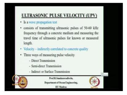
So we will see one by one what are the different types of test, what is the procedure. This is a wave propagation test. What we do in this, we transmit the ultrasonic pulses in this frequency, 50 to 60 kilohertz frequency and we pass it through a concrete medium. Generally this is used for concrete structures and what we basically measure is the travel time of ultrasonic pulses for known or measured length. So we should know the thickness of the concrete specimen.
