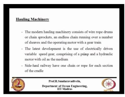
The hauling machinery consists of wire rope drums, (spine) chain sprockets, endless chain running over a number of sheaves and the operating motor with a gear train. Then we also use
