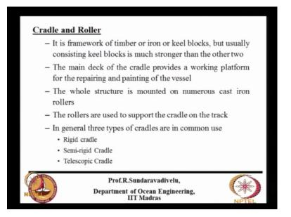
The cradle and roller is a framework of timber or iron or keel blocks but usually consisting keel blocks is much stronger than the other two. They can have cradle with a keel block also. The main deck of the cradle provides a working platform for the repairing and painting of the vessel. So when they take the platform with the, when they take the ship with the cradle, they will keep the ship in the cradle itself. So each ship will have a separate cradle.
