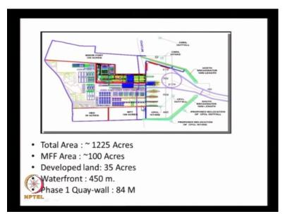
This shows the layout of the breakwater. This is north breakwater, this is south breakwater. This is a container facility. This is a shiplift facility. These are the other structures. Total area is 1,225 acres, whole area. That is called as modular fabrication facility, that is MFF, that is 100 acres. They have developed the land of 35 acres with very strong foundation. The waterfront required is about 450 meters. The phase 1, they have built one quay-wall also somewhere here.
