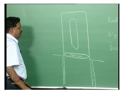
What dry dock, what they are asking is, I am drawing the plan of the drydock. So the vessel will be kept here like this. Dry dock, this is the plan of the vessel, then we have a gate. Gate is like this. What they are asking is a lead-in-jetty, there is a jetty here. On both the sides also it will be placed. So this is, there are different types of gate, this is called as floating gate. When they ballast, the gate will go and sit here.
