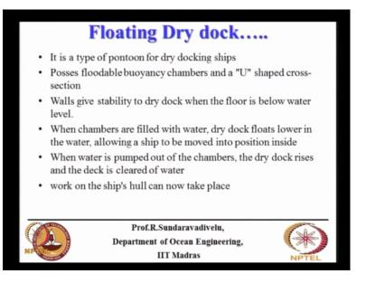
So it is a type of pontoon for dry docking ships. The chamber shape is typically U shaped. These walls give stability to the dry dock when the floor is below the water level. When the chambers, that is chambers are filled with water, dry dock floats lower in the water allowing a ship to be moved into position inside. When the water is pumped out of the chambers, the dry dock rises and the dock is cleared of water. Work on ship hull can now take place.
