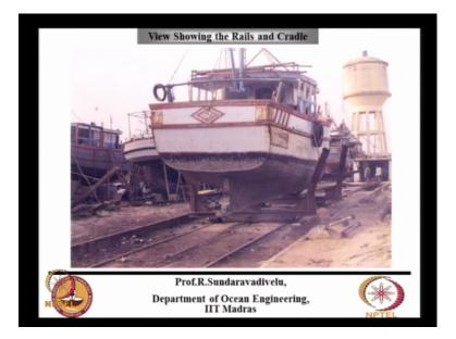
This shows a conventional ship repair. This is not a ship, this is for a floating vessel. This is in a place called Dhamra in Orissa. So here you are seeing the two rails. These are the two rails. I think these are the two rails I think. These are the two rails. This is another structure. This is what is I am talking about the cradle. This is a keel portion of the vessel. They will be pushing, this is a very simple structure because this is a very small boat facility.
