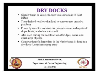
Is a narrow basin or vessel flooded to allow a load to float inside, then drained to allow the load to come to rest on a dry platform. That is first allow the vessel inside with water inside, then remove the water. This can be used for construction, maintenance and repair of ships, boats, and other watercraft. There is a regulation that once in 5 years the under keel of the ship has to be checked. For that reason we have to drydock the vessel once in 5 years.
