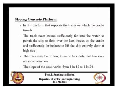
This sloping platform supports the tracks on which the cradle travels. The track must extend sufficiently far into the water to permit the ship to float over the keel blocks on the cradle and sufficiently far inshore to lift the ship entirely clear at high tide. That is one ship should float, one ship length of slipway platform is required where the ship will float. But another length is required where the ship will rest on keel block and bilge block.
