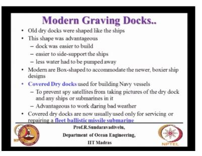
Olden day the dry docks were built like shape of the ship. The shape was advantageous because dock was easier to build, easier to side-support the ships, less water had to be pumped out away. But modern dry docks are box-shaped as they have done here. We use covered dry docks for navy vessel. This is mainly done to prevent the spy satellites from taking pictures of the dry dock and any ships or submarines in it.
