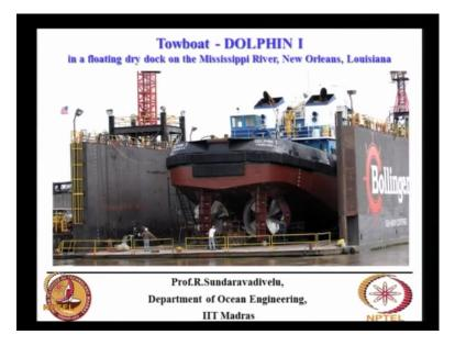
This figure shows the floating dry dock. These are the side walls of the floating dry dock. This is the bottom chamber. You can see the person standing here. There are different sections. This is one typical section which will have its own machinery. Then like this there will be at least about 5 sections. And when you ballast this, when you put water into this, the whole floating dock will go down and then this vessel also will go down.
