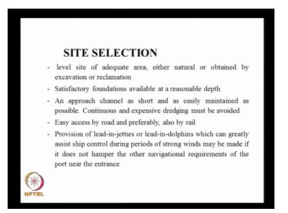
So site selection is very important and satisfactory foundations at reasonable depth should be available. A short approach channel is preferred. Dredging both capital and maintenance should be as minimum as possible. There should be easy access to road as well as for rail. You have to provide some lead-in-jetties, lead-in-dolphins which can greatly assist. Ship control during periods of strong winds and other navigational requirements, these are the requirements for a dry dock.
