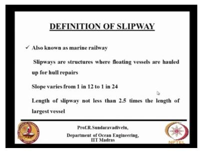
Definition of slipway, this is also known as marine railway. They are structures where floating vessels are hauled up for hull repairs. The slope varies from 1 in 12 to 1 in 24. So this slope is very important. A steeper slope, the hauling power required will be higher. Flat slope, the distance required into the water is larger. That is the length of the slipway, is generally about 2.5 times the length of the largest vessel that is to be hauled.
