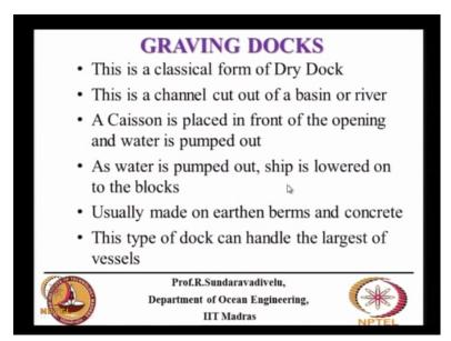
There is what is known as graving dock. This is nothing, this is a classical form of dry dock. You cut a channel from the basin of the river. A caisson is placed in front of the opening and water is
