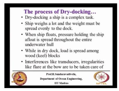
So very complex task. Ship weight is very high. The ship weight must be spread evenly on the dock floor. Hello! Who is talking there? Do not talk. When ship floats, pressure holding the ship afloat is spread throughout the entire underwater hull.
