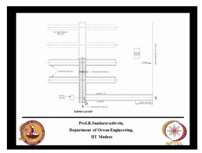
This is one typical system where the transfer cradle is used. So this is the main slipway. This is the river. This is land area. This is a winch house here. They push the vessel here like this, then they transfer it like this right up to the end. We have the tracks on either side of this, transfer track. And these are called as repair tracks. This they want to do it in future.
