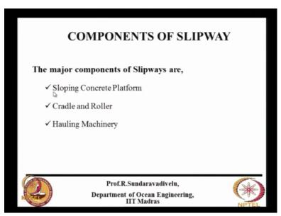
The components of the slipway, these are the three main components. One is a sloping concrete platform, that is a cradle and roller, then there is a hauling machinery. These are the three main components for a slipway.
