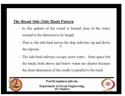
The broadside pattern, the vessel is hauled clear of water normal to the direction of its length. That is, for the side haul it moves the ship sideways up and down the slipway. The side haul railways occupy more water, front space but the tracks both above and below water are shorter because the short dimension of the cradle is parallel to the track. That is cradle width will be lesser.
