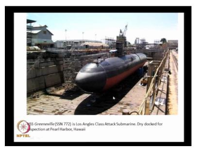
This photograph shows atomic submarine. You can see the space what is given here on either side of it. This is a dry dock. There are some cranes here which will lift some of the components from this side. There is a staging which is given here so that you can access any part of the submarine. Typically the height is about 1.5 meters, so somebody can go below and do the work also.
