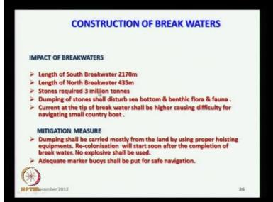
So when you want to construct the breakwater, southern breakwater is about 2 kilometre, North breakwater is about 500 metres, the stones required are about are about 3 million tonnes with artificial armour. Now it has gone up, about 6 million tonnes with breakwater. When you dump the stones, they will disturb the sea bottom and benthic flora and fauna, current at the tip of the breakwater shall be higher causing difficulty for navigating small country boat.
