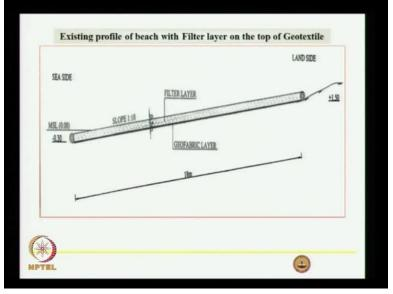
Next you place the filter layer that is 150 mm thickness. Up to 150 mm size, 300 mm thickness, you maintain the slope of 1 is to 10. Suppose the slope is flatter than this, you may rise it to make it 1 is to 10. If it is steeper also if it is steeper, you fill it and rise it. If it is flatter, you make it as it is. You do not make it slope 1 is to 10. Suppose it is 1 is 220 slope is there, you leave it as it is. Do not try to make it 1 is to 10. But you adjust in the core layer.
