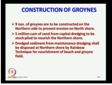
And to keep the artificial nourish the sand in place, we are planning about 9 groynes. Now we have increased it to 11 and about 5 million cubic metres will be nourished on the northern side as the stockpile and further when you do the maintenance dredging, we will use it by rainbow technique to the northern side.
