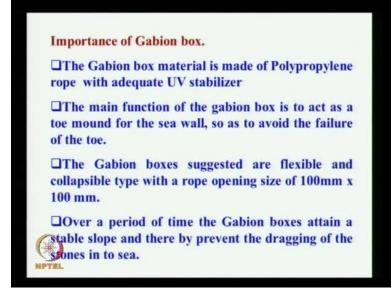
So the gabion boxes these are also made of polypropylene rope, they are having adequate UV stabilisation. UV stabilisation means they will provide some colouring is there, some black colour, some dark coating or something like that they will do. But there are different type of gabion boxes, one is made of metallic wires, another is made of rope. We prefer rope because it is flexible and adjust to the seabed.
