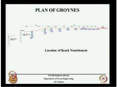
This is what is actually now being built now. These are the inlet groynes, these are the 11 groynes. The distances are shown here. This is the seawall which is shown here. These groynes are built 50 percent now. Now they will be stockpiling the sand right up to this toe of the breakwater.
