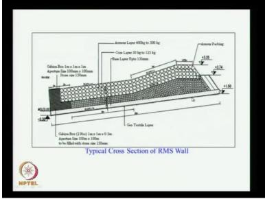
This shows the typical cross-section of the rubble mound seawall. We are given mean sealevel as 0.0. This is not a normal convention. In short data means given as 0.00 but here we have used mean sealevel as 0.00. So we can take about 30 centimetre below the mean sealevel you have to take. Typically, the seawall width is about 18 metres, that is from this point to this point is about 18 meter and we give a slope of 1 is to 10.
