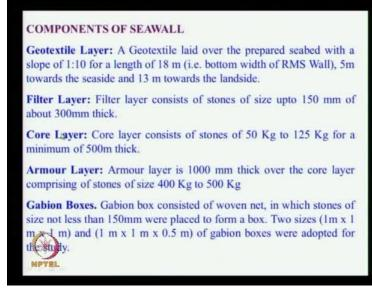
So these of the components of a seawall. One is a geotextile filter, the other is a filter layer, 3rd one is a core layer, a normal layer and gabion boxes. So this is in a slope of 1 is to 10 and about 5 meter towards the seaside and 13 meter towards the land side. The 5 meter towards the sea side is from the high tide level to the toe that is about 5 meters. The filter layer consists of stones up to 150 mm of about 300 mm thick.
