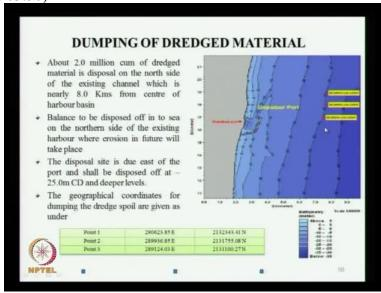
And we have shown the locations where this dredge material will be dumped. So 2 million cubic metre will be disposed on the northside of the existing tunnel which is nearly 8 kilometres from
