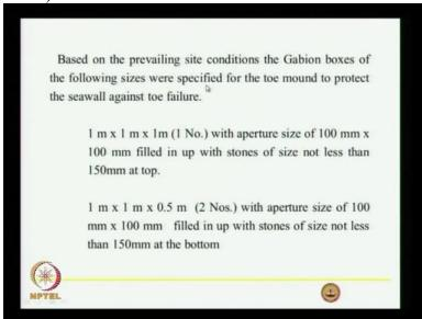
Then we have the gabion box. The cost of 1 metre by 1 metre by 1 metre box will be around 1500 rupees and this is the size of the opening, 100 by 100 filled with stone of not less than 150 and another size is 1 by 1 by 0.5.
