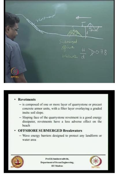
Suppose you have a shoreline going like this, then this is your water level. Revetment means you put some structure on the slope. This is called as the revetment. And when you talk about the offshore submerged breakwater, this is some kind of a structure which we built below the water level. So whenever the wave is travelling from Seaside to the land side when it comes over here, the wave will break here.
