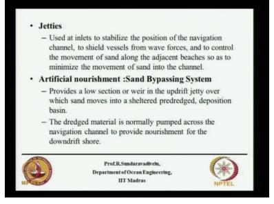
Then we have jetties. These are used as inlets to stabilise the position of the navigation channel. They are used to shield vessels from wave forces and control the movement of sand along adjacent beaches so as to minimise the movement of sand into the channel. Jetties are built mainly at the inlets. Then we have artificial nourishment. This artificial nourishment is done by the sand bypassing system.
