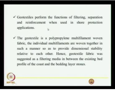
What are the functions of various materials we have used? One is the geotextiles, they perform the functions of filtering. Filtering means allowing the water passage. Separation between the seabed material and the filter material. It acts also like a reinforcement when used in shore protection. If you put a geotextile filter, the whole mass above the geotextile filter acts as a single unit.
