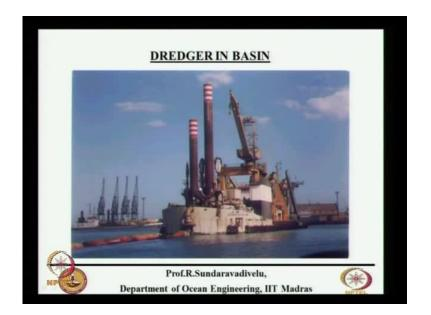
Normally they use a dredger to dredge the basin and there is a pipeline here. Initially what they want to do is, they want to nourish the portion between this existing breakwater for the inlet and the 1st groyne by laying a pipeline. Other thing, they will go into the sea here by another dredger and then do a rainbow. I will have a slide, I will show that. So they are dredging and there is a floating pipeline.
