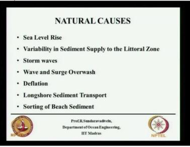
So we will list the various natural causes. One is the sealevel rise. They say the sealevel is rising. It varies from 1 millimetre to 100 millimetre, that is the range they are telling per annum. It is not yet quantified. The variability in sediments apply to the littoral zone. The sediment is coming from the rivers when there is a sediment is there, there are various sources. One of the source is the sediment coming during floods from the river.
