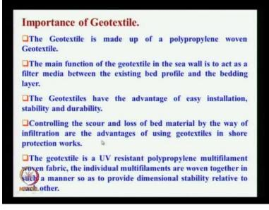
This geotextile is made up of polypropylene woven geotextile. Main function is to act as a filter media. Filter media means like our coffee filter only. Between the existing bed profile and the bedding layer. Bedding layer is nothing but the filter layer. It allows water to percolate but it does not allow the seabed material to get into the bedding material. Bedding material is a filter material, either a sand or a stone of size up to 150 mm. So these 2 things should not come in contact.
