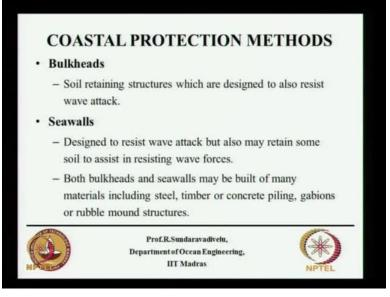
There are various methods that are used for coastal protection. One is called as the bulkhead, another is a seawall. Both bulkhead and seawalls are constructed parallel to the shoreline. Bulkheads, they are retaining the soil. Whereas seawalls do not retain the soil. They both are designed to resist the wave attack. There are many materials that are used for building the bulkhead and seawall.
