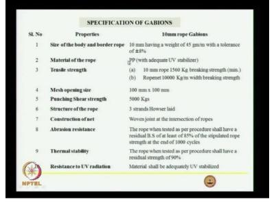
This is for the gabion box. This weight is 45 grams per metre. This is a polypropylene rope. The breaking strength is given. Mesh opening size is given, punching shear strength, the type of the rope, abrasion resistance, thermal stability, resistance to UV radiation. Normally they claim, it is resistant for about 10 years, 15 years, 20 years like that. Actually it will not fail. Maybe the strength will reduce by about 40 percent over a period of time.
