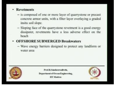
Revetments, this on the beach itself you put some filter layer and then put some armour units. This is called as a revetment. So this revetments also is a energy dissipator. They have less adverse effect on the beach. We have one more concept that is called as offshore submerged breakwater. These offshore submerged breakwaters are built in the sea and they act as a wave energy barriers and protect the landform or water area. So let us see by sketch all the different types.
