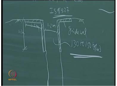
This is called as the grid wall. So this is your ground level, typically this goes for about 2.2 metre it will be for 2.2. Or it can be 1.5 by 1.5 also. So this grid wall is given in terms of cubic metre. Then the excavation is also done in cubic metres. Whatever is the excavation quantity will be the concreting quantity, that also will be given. Then we have the steel. There are different grades of steel. 415 can be used or 500 can be used depending on the type of steel.
