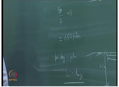
Let us say length of the length is about 900 metres divided by 7 into 5 approximately about 650 piles. This piling gantry with 5 rigs approximately we can do per day at least about 3 piles. Then you need about 220 days for driving 650 piles. So this per day if we can make 3 piles, to make 650 piles we need 220 days. Once you are completing the pile, you can bring the deck system from behind and then start doing the operations.
