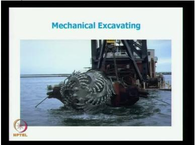
Then, this is another mechanical excavator, a cutter section dredger with teeths here. It is used for rock dredging.
