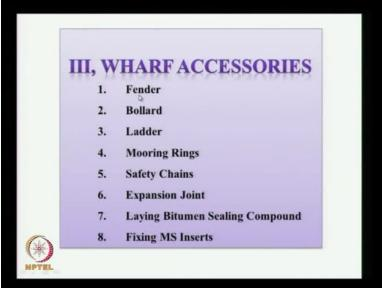
Then we have the wharf accessories, the 3rd system that is the Fender, Bollard, ladder, mooring rings, safety chains, expansion joint, the expand joint, laying bitumen sealing compound and fixing of MS inserts, this is either for conveyor system or for cranes, this is insert (())(30:43). So these are the various wharf accessories. This we have to design and accordingly we have to provide this in the estimate for various items.
