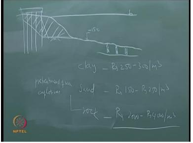
This is done by explosives. So we will lower the explosives in pre-drilled holes. Suppose you have the rocky strata here, what they do is, they drill some holes. This is your water level. They drill the hole through this, they lower the explosives here and then they blast it and then they loosen the rock, then they use the cutter to remove the rock. So in that case, the cost will go up to Rs. 4000 per cubic metre. These are the various methods by which we do it.
