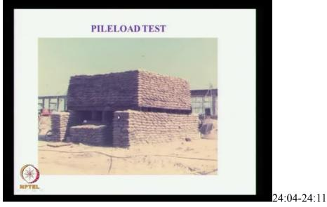
This is a similar this is some procedure for doing the pile load test. So here what we have done is, we have put the weight required. Suppose the capacity of the pile is 400 tonnes, we have to test it for 1.5 times 400, that is 600 tonnes. You stack the weight of 600 tonnes and use a below and then apply the load. Otherwise you can test this pile and use this as a reaction pile, that is also possible.
