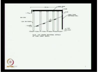
This shows a typical berthing structure. The dredge level is minus 15. There are 1, 2, 3, 4, 5 rows of pile and here we have the diaphragm wall.Ground level is somewhere here at this point. Originally, the whole structure can be built on land and then you can dredge or you can build only the breakwater on land, other things if they are already dredging is carried out, we can do this construction. Stone pitching is required if the diaphragm wall design has to be optimised.
