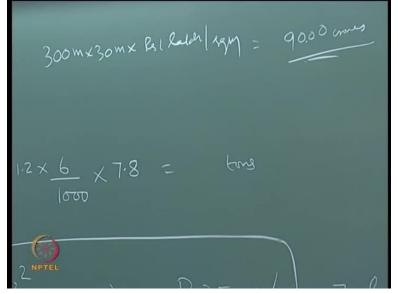
One more block cost estimate is there. Suppose the berth size is 300 metres by 30 metres approximately the cost is about Rs. 1 lakh per square metre. That means this will be about 90 crores. This is the approximate cost for a typical berth of length 300 metres and width 30 metres, the approximate cost will be 90 crores.
