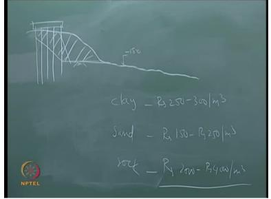
See this, there is a project in Cochin where they were building a structure on the land, this is the structure which they want to build it somewhere here, the berth will be built here. Then afterwards, they will dredge it up to this level. This is the dredge level which is required, minus 15. They will remove the soil subsequently. When they started removing the soil subsequently like this, this does not form a slope like this. This was forming a slope like this.
