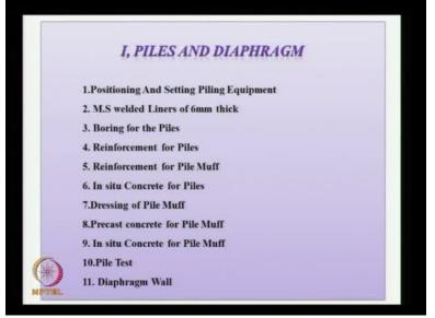
Now we will go section by section. 1st section is the piles and diaphragm wall. We have to 1st position and set the piling equipment. Then we have to make the liner for the pile, then we have to bore through the liner into the into the soil up to reaching the founding level. Then we have to tie the reinforcement, keep it ready and lower it into the bore. Then we have to make the reinforcement for pile muff and do the concreting either in situ or precast.
