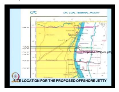
This is taken from Naval hydrographic chart and this line shows 10 meter contour this line shows 20 meter contour that means the water depth is around 20 meters and this line shows 5 meter contour and this is your shore line. The distance to 5 meter contour is very small here compared to many projects and I will show an enlarge figure later on. This is for the coal terminal facility what is planned here.
