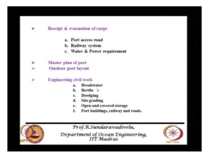
Then we classify the works into two categories Civil works and Mechanical works the civil works are generally break waters berths, dredging, side grading, open and covered storage shed, port buildings, railway and roads. These are the major components of Engineering Civil works.
