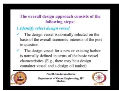
So what are all the design approach for this channel design. First you have to select the design vessel. So design vessel is based on the overall economic interest of the port in question. So when we want to select the design vessel you should see for a type of cargo what is a majority of the maximum share of the cargo in what size of the vessel it is being
