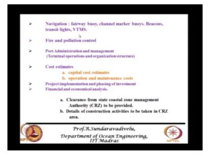
Then we have navigation where a buoy channel marker buoys beckons, transit lights, VTMS. Now what is VTMS any idea vessel traffic management system. This moves just like air traffic controller there will be a vessel traffic controller will be there it is not in place in Indian ports but this is very much required. So every day if you are getting around 10 vessels, you have to manage how to bring these vessels and take these vessels out.
