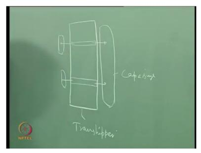
Transhipper is a just like a ship with some crane facilities then you bring the vessel on one side bring small badges which are coming from rivers in Goa. So there will be cranes here which will take the cargo from here and load it here. So this may be a cape size vessel which the Goa port not be handle will not be able to handle so they will put a transhipper here and go to 20 metre contour or 30 metre contour. This is being practiced now.
