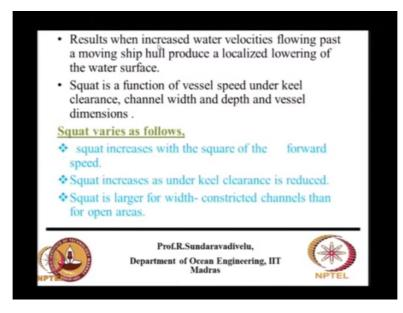
So when increase water velocity flowing past a moving ship hull produce a localized lowering of the water surface. Squat is a function of vessel speed under keel clearance, channel width and depth and vessel dimensions. And squat varies with the square of the forward speed. So the speed is more, squat means how much clearance got reduced.
