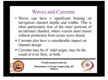
Wind also has significant impact but the waves can have a significant bearing or navigation channel depths and widths. So this is mainly for router portion of the entire channel where vessels must transit without protection from motion wave attack. Current also have a considerable impact. Currents can be of tidal origin may be the result of river flow or both. River flow means it is from the river to the sea, tidal means it can be into the river out of the river.
