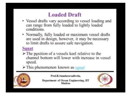
So the vessel draft can be fully loaded or lightly loaded conditions, so you normally take the fully loaded. Sometimes we have to limit drafts to a shore safe navigation. That means we may not load the vessel for the full load to aid navigation. For example (if the berth is) if the port is designed much earlier and it cannot take higher draft, but you cannot go and check the vessel because there is a particular type of vessel which is most commonly used for a particular type of cargo.
