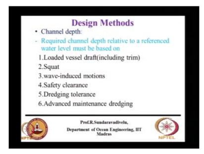
Some ports do not carry out this advance maintenance dredging, but we normally recommend this advance maintenance dredging. We are designing a floating doc in Port blare. The floating doc is kept by the side of the berth. The floating doc is maintained once in 5 years. So below the floating doc for 5 years we do the advance maintenance dredging, because the floating doc will be in the same position for 5 years.
