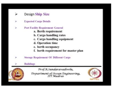
The first parameter is the Ship size it is the Design ship size there will be various ships that will be coming to the berthing facility. What are the different types of ships? Hmm? panamax, kape size, any other type of classification? Containers and tankers. So you have to decide suppose you are using general cargo container and bulk cargo and tanker for each one of them you have to give the size of the ship whether it is a panamax or;
