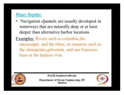
So we have to develop the natural channels and waterways that are naturally deep or atleast deeper than alternate harbour locations. This is how you have to decide that means suppose now a days we have to bring the vessel about 12 meter draft and 14 meter depth is required. Normally what we say is about 10 meter water depth what distance it is available from the shore, because 4 meter you can reach.
