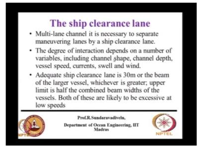
So for multi channel you have to separate maneuvering lanes by a ship clearance lane. So this degree of interaction over matured provide it depends on the channel shape it can be straight or it may be curved what is the depth of the channel? What is the speed of the channel? What is a current? Swell and wind. What is a vessel speed normally inside a harbour basin when you want to bring in.hmm? how much?
