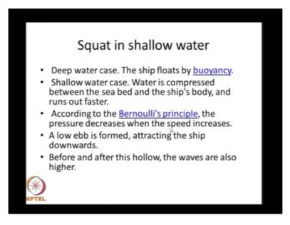
So in deep water case the ship floats by buoyancy shallow water, water is compressed in the sea bed and the ship's body and runs out faster. So there is a effect of bottom here, so in shallow water this water between the ship bottom and the sea bed is compressed and flows faster. According to the Bernoulli's principle the pressure decreases when the ship speed increases.
