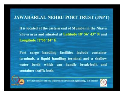
Then we will see next JNPT. Jawaharlal Nehru Port Trust is the latitude, longitude is given. This port is handling mostly container and we also have a liquid terminal we also have shallow water berth, where we use the break-bulk and container traffic. Break-bulk means coal, iron ore and things like that, but mostly JNPT is handling only container traffic. (30:08)
