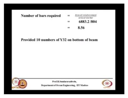
That is other type of design, so normally whatever reinforcement that is coming for stress level check you have to increase at least 30 to 60 percent to check for crack width, I will explain the crack width later.
