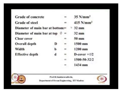
What is the maximum diameter of bar available? 32, I think 36 also available then you provide clear cover 50, the depth of the beam is 1500 width is 1200. Generally the width of the beam in harbour constructions are much much wider compared to any other thing.
