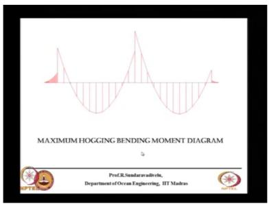
This shows the sagging moment the bending moment is maximum here it depends on the load condition where you are placing the load and this shows the bending moment envelop what you are trying to get. Considering all the load combination what will be the maximum bending moment. If you are able to get this bending moment envelope properly then you can provide the reinforcement accordingly.
