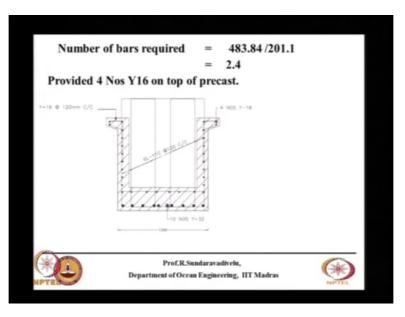
You calculate the number of berths and provide adequate berths like this. if you want to take the full width of the beam 1200 you need this shear reinforcement coming from the precast portion also into the incetive portion, you have to tie it together. You cannot assume the bond the interface bond between the precast and incutive construction. You need reinforcement and carriage into the precast and incetive that is done by this shear stirrups.
