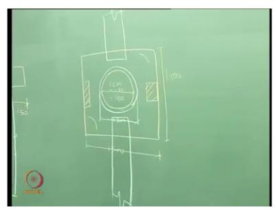
Suppose the pile is 1200 millimetres the pile cap what you are making will be like this, this is a pile which is coming here and this dimension will be 1500, 5500 and this pile cap is made to rest on the cover portion of the pile. So this is your 1200, generally the cover is 75 that
