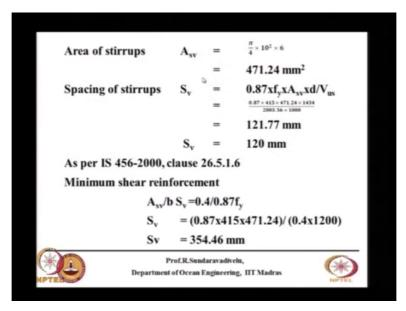
You calculate the area of stirrups and then what you do is, you calculate the spacing it is coming 121.77 you provide a spacing less than this 120 millimetre centre to centre. This also should not become very close, generally the shear stirrup spacing is about 100 millimetres not
