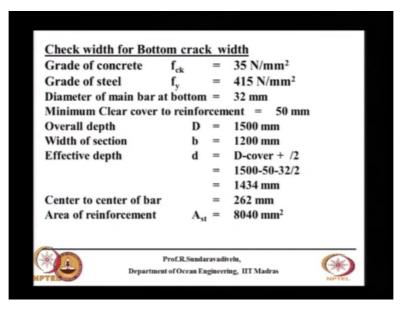
You cannot leave the skin like this. This is called as the side face reinforcement. The side face reinforcement also about some minimum percentage is there that is 0.05 times sectional area that you calculate
