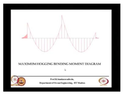
There are two types of bending moment one is called as a hogging bending moment another is called as a sagging bending moment. What is hogging bending moment? What is sagging bending moment? Hmm? Sagging is compression on the top, hmm that is the way to answer you take the compression at the top and tension at the bottom that is called as a sagging moment, hogging means uhh you can say about convex and concave also.
