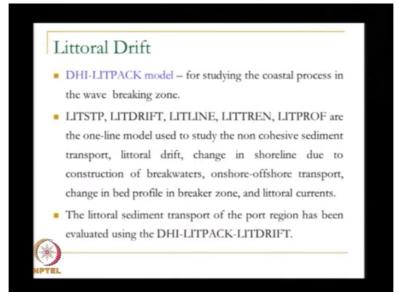
The next model is literal drift this is very important for shore line evaluation that is the third study which I have written here. This is developed by one institute called Danish Hydraulic Institute. We will be using this model for finding out the shore line changes. The shore line changes occur due to construction of break water on shore – off shore transport change in bed profile in breaker zone and literal currents. These are the various requirements.
