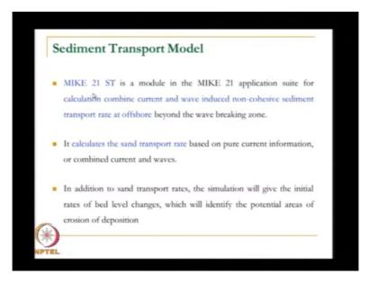
We use software called Mike 21. This is used for calculation of combined current and wave induced, non cohesive sediment transport rate at offshore, beyond the wave breaking zone that is the capability of this model. Basically you want to study how much sediment will be disturbed.
