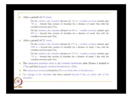
After 10 years; To summarize the maximum accretion close to the southern break water of 25 years is limited to 170 metres and that along the southern break water is 120 metre. So what they are telling is this is 170 metre and this is 120 metre. Maximum erosion is limited to 25 metres on both sides of break waters.
