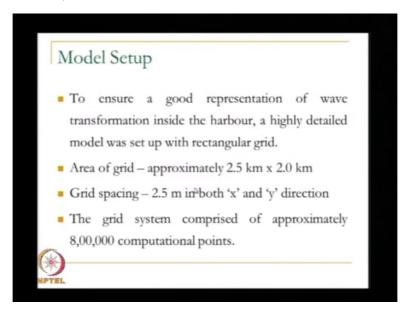
Whenever you do this type of modelling one of the main requirement is what is the area you are taking for the study, here we are taking 2.5 by 2 kilometre. Suppose you do not take the area properly then also the model will fail. The second one is what is the spacing of the grid points that should be 2.5 metre is a fairly closed grid which you are using. And we have 800000 computational points within this grid.
