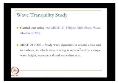
So these are the two studies which we have done one is the sediment transport and the dredge disposal. The next study is wave tranquillity study. So you are supposed to know about this elliptic mile slope wave module this equation is there which is used to solve this problem. So we have to study the wave tranquillity for a single wave height, wave period and wave direction.
