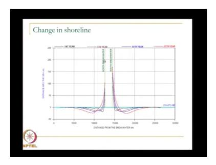
So this shows the result what is happening this is your shore line of the coastal line and this has been developed for about 250 metre into the sea. Here the distance from the break waters are shown these two are the north and south break waters they are extending for about 2 and half kilometres. Each break water is going for about 2 and half kilometres. But we are showing only 250 metres and here we are showing first year fifth year tenth year and twenty fifth year.
