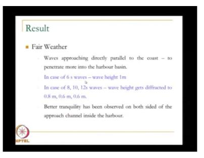
For 6 seconds waves all the waves are (())(22:33)same as 1 metre. But higher period waves when it goes inside the wave height become lesser. The better tranquillity has been observed and both side of the approach channel inside the harbour. This is approach channel so when either side of this we have better tranquillity. So this is about the south west monsoon and north east monsoon.
