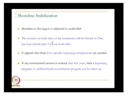
So what is to be done for the shoreline stabilization? So we do not need a bypassing arrangement. Bypassing arrangements means you remove the sediment from the southern side and put it on the northern side so you do not need this. If anything is seen then we can go for a bypassing program.
